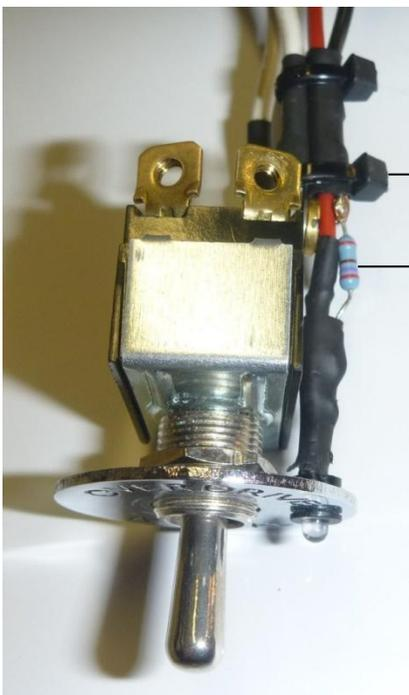
LED is insulated and zip-tied to switch wire. This makes it rigid enough to protrude into the holder and stay there.
